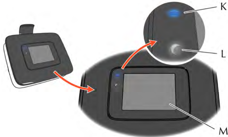
(K) Battery LED - lit when battery is charging, (L) Standby LED - blinking in Standby/Sleep mode, (M) Touch panel Display
